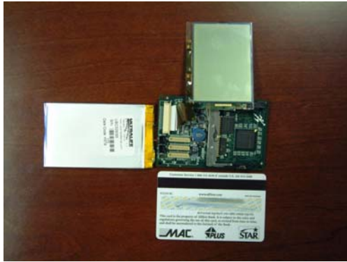
Figure 4 The prototype UPTD without casing and buttons; clockwise from the left there is 1) the battery, 2) the display, 3) the SBC and CF slot, 4) a credit card that indicates the UPTD dimensions.
